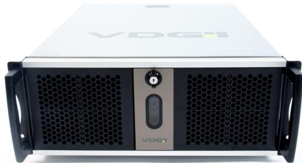
The front-mounted hard-drives are configured for hot-swapping, as are the cooling fans, to ensure 24/7 operation. This means that they are easy to service and can reduce running costs. The reliability is ensured through a standard RAID 1 configuration for OS redundancy, and RAID 5 configuration for data redundancy, but can be configured otherwise if necessary. Redundant power supply included.
