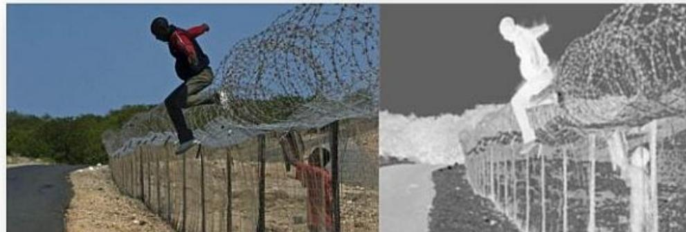
*FenceGuard: Perimeter intrusion detection*
