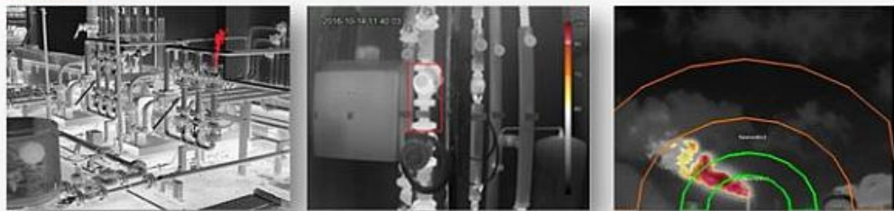
Fire detection, hot-spot and flare monitoring
