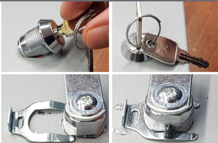
Insert the lock with the lip in the recess and secure this with the supplied fixation slide.
