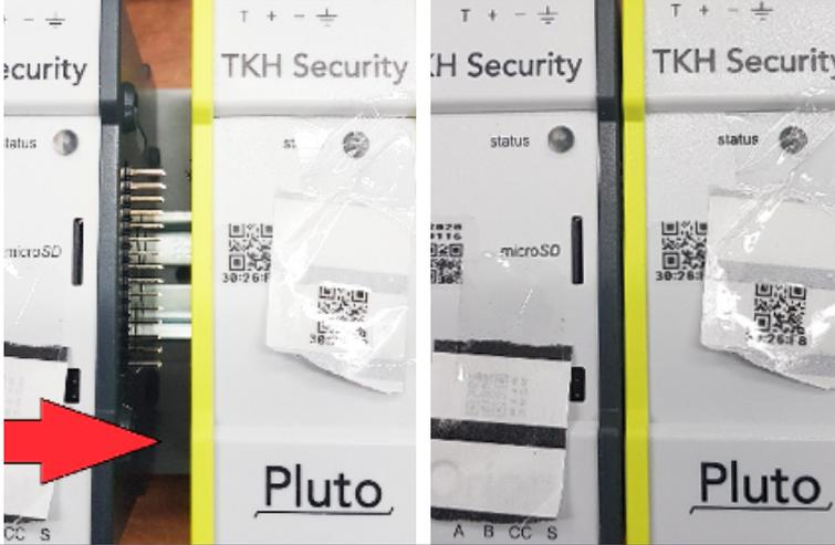
In this step, you press the Orion door controller to the Pluto network controller, or another Orion door controller. You need to repeat this step, if more door controllers need to be connected.
